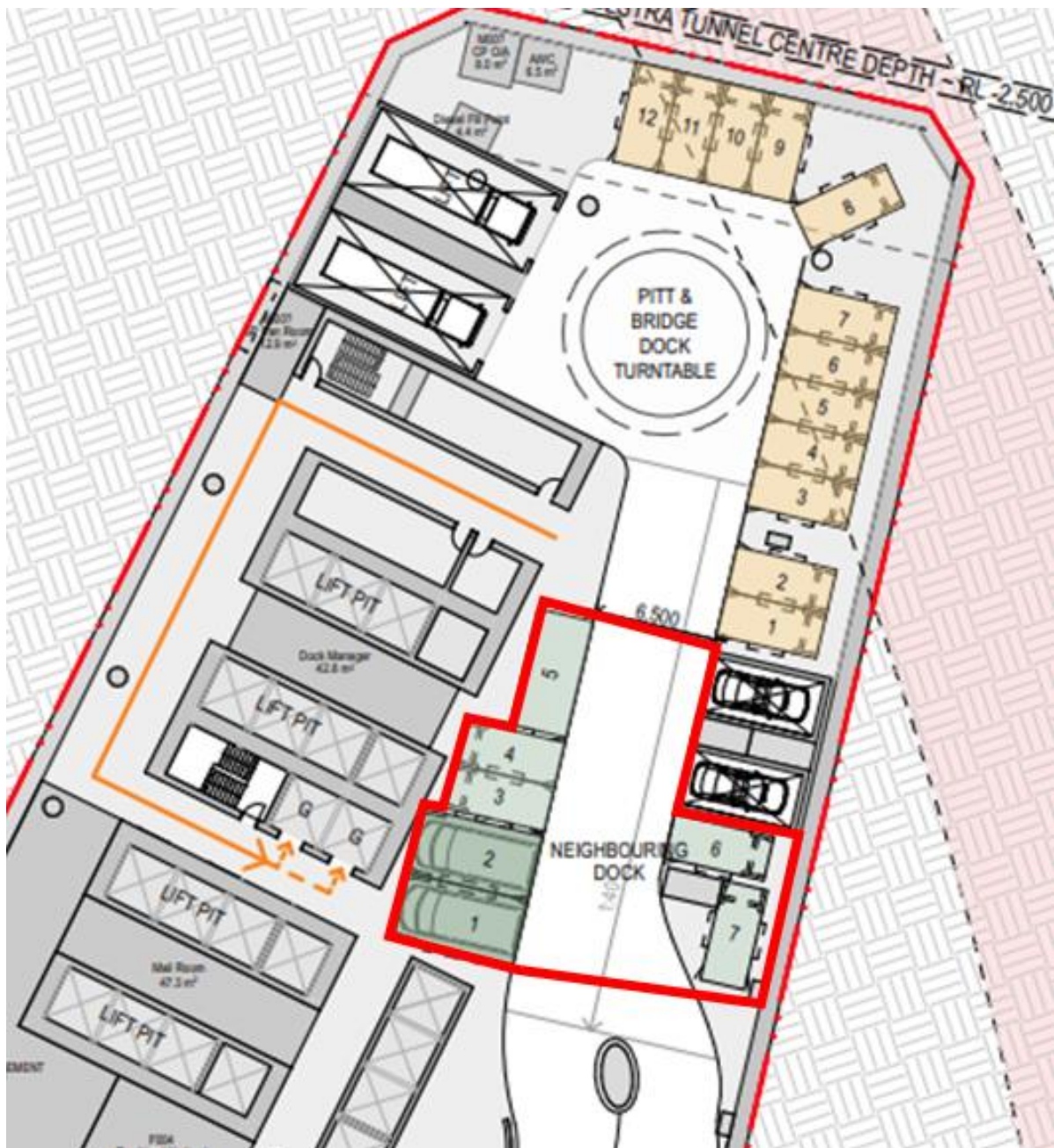
Figure 6.2: Loading Dock Layout
